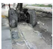
The best material found to date is a lightweight, crushable concrete, the FAA said. When an aircraft
